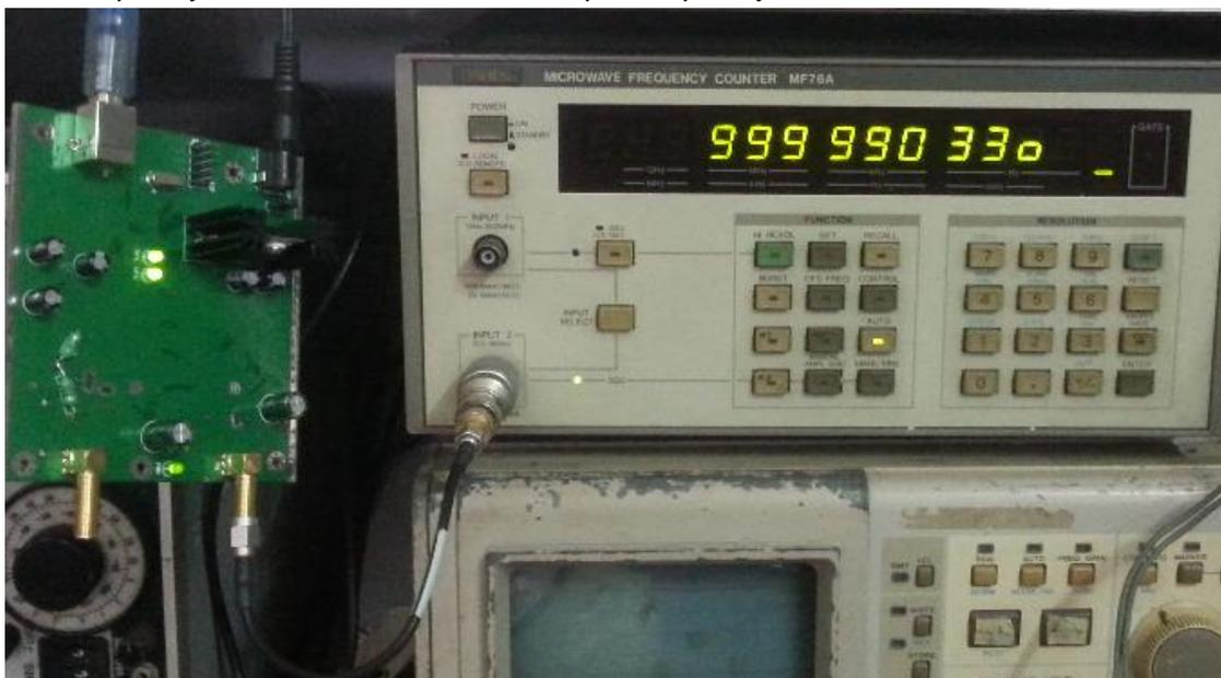
Test output frequency in this case 999.990 330MHz
